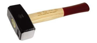
Features & Benefits  $\sim$  Drop forged high carbon steel head  $\sim$  Hardened & tempered for superior strength and durability  $\sim$  Black lacquered to protect against corrosion  $\sim$  Traditional ash shaft  $\sim$  Weight: 1500 g / 3.1/2lb
